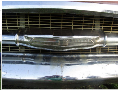
57 Chevys had a plastic insignia that often times broke. This is a rare aftermarket replacement that bolted over the cracked insignia on the grille bar.
